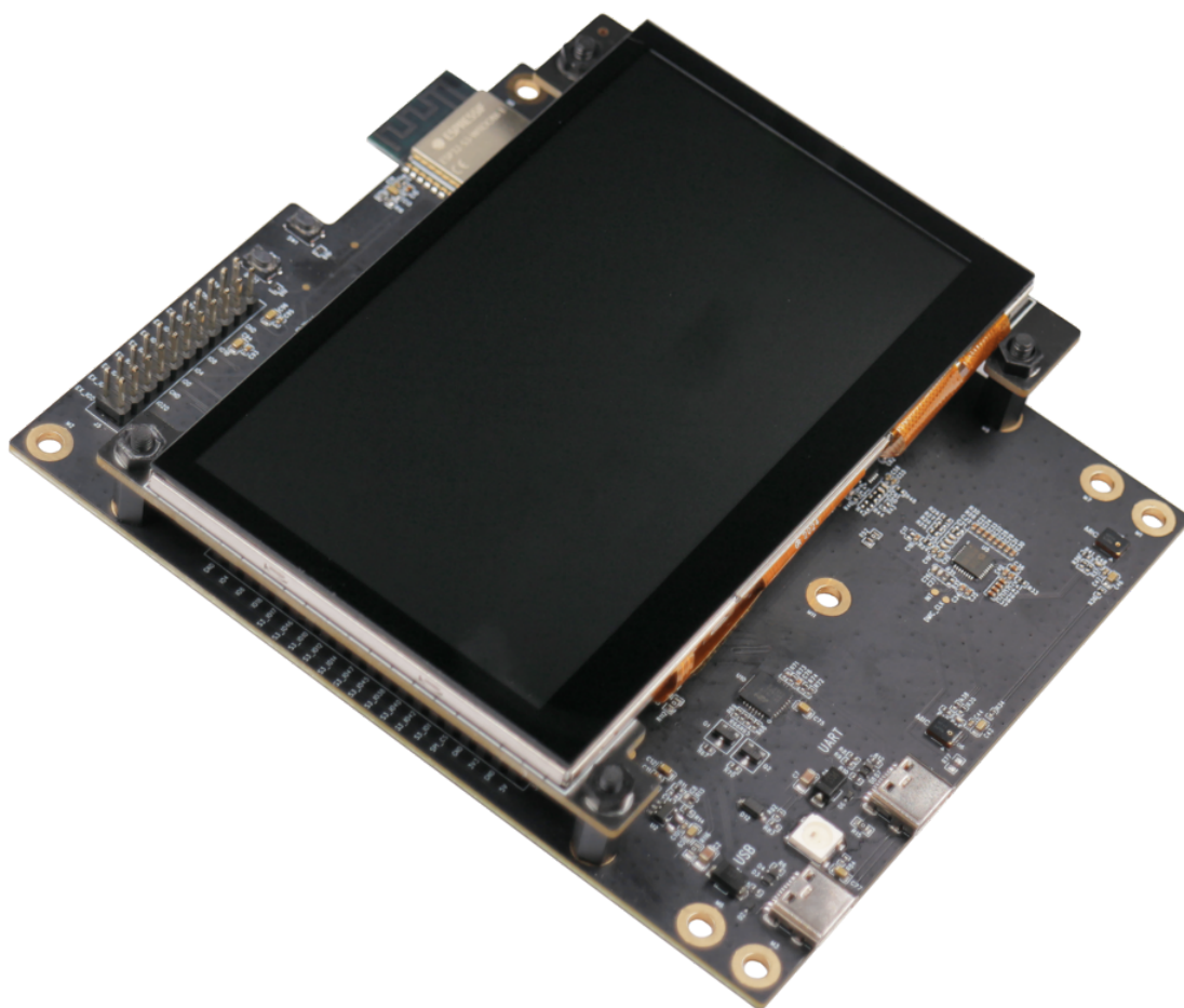
Fig. 20: ESP32-S3-LCD-EV-Board-2 with 800x480 LCD
