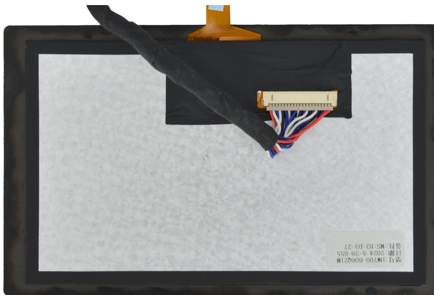
Figure 26 Connect LVDS screen cable to LVDS screen
